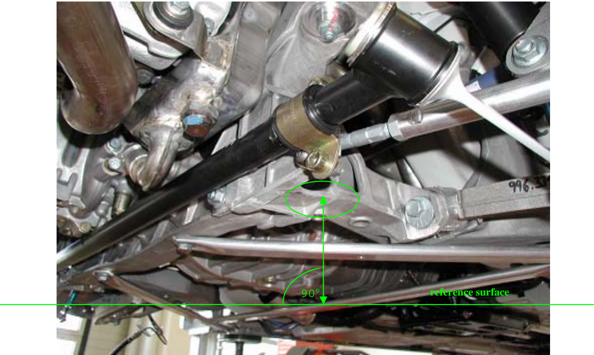
RIDE HEIGHT MEASURING POINT - REAR AXLE
